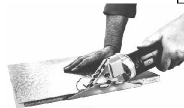
flush trimming of projecting edges with side guide
